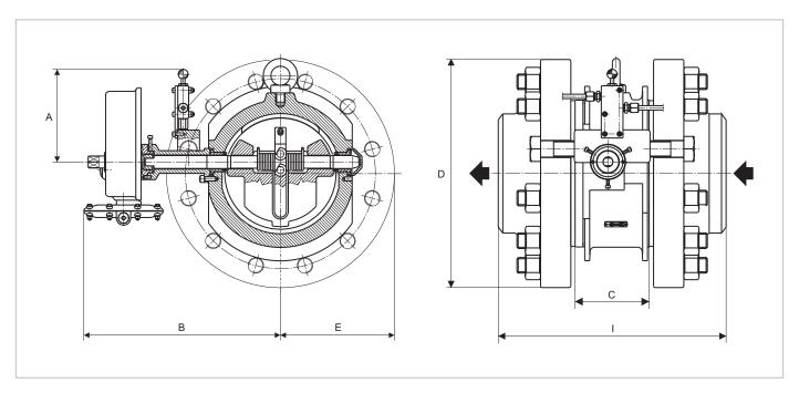
Figure 5. BM6X Series Dimensions
