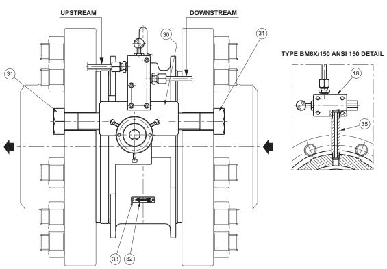
Figure 9. BM6X Series Slam-Shut Valve DN 80/100/150 Casting Version
