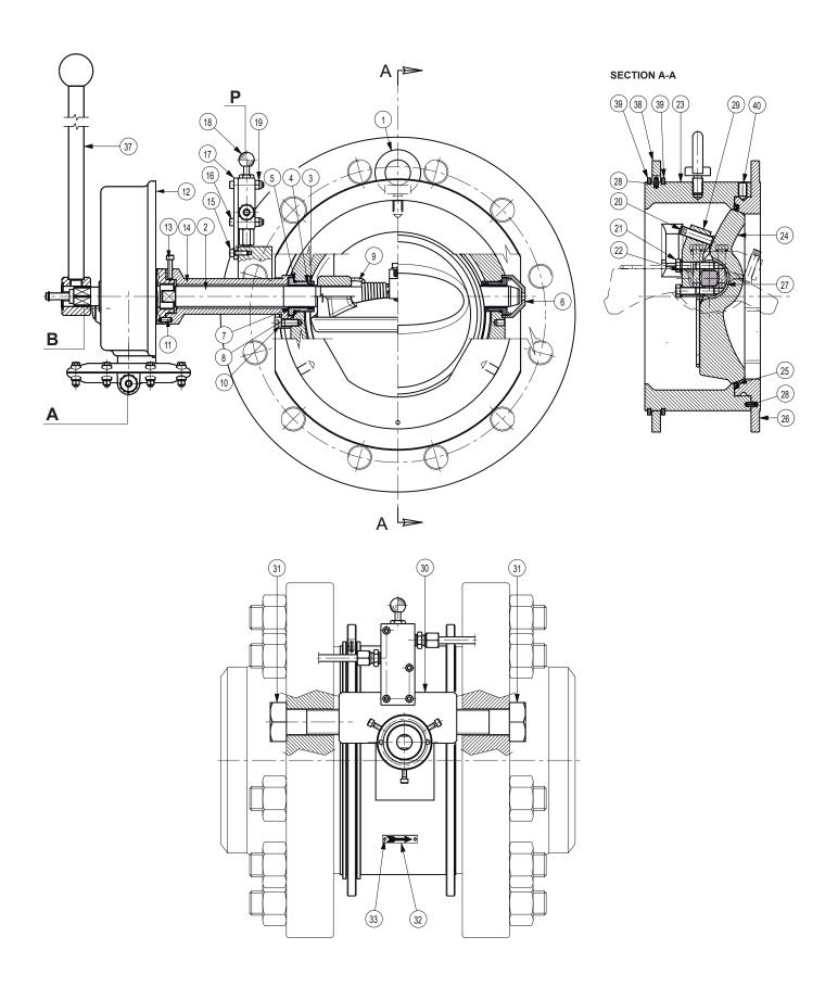
Figure 10. BM6X Series Slam-Shut Valve DN 200/250/300 Machined Version
