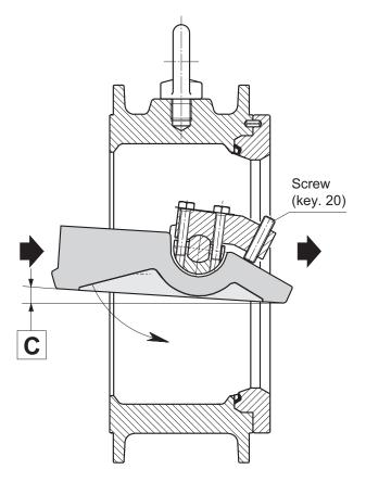
Figure 8. Type BM6X Shutter Position
