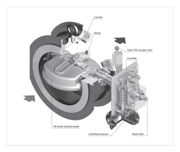
Figure 6. BM6X Series Operational Schematic
