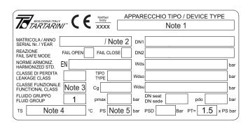
Figure 2. Label for BM6X Series Slam-Shut Valves
