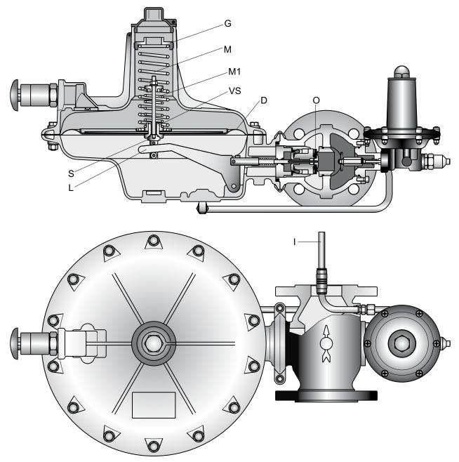
Figure 5. A/140 Series Operational Schematic
