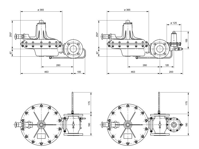
Note: The regulator can be installed with vertical or horizontal orientation of the actuator. \* In high pressure versions (AP), this dimension must be increased by 100 mm.
